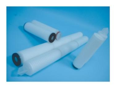
ExPleat PFH Series are designed to meet the special needs of the electronics and high-purity chemical industries. Polytetrafluoroethylene (PTFE) membrane is resistant to virtually all chemicals. Because of the hydrophobic nature of PTFE, it can also be used to filter process gases. To minimize extractables, each cartridge module is pre-flushed with 18 Megohm-cm DIW.
